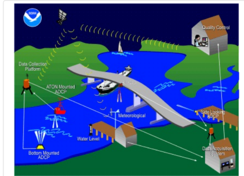
An example of the sensors that make up the Physical Oceanographic Real-Time System (PORTS®).
